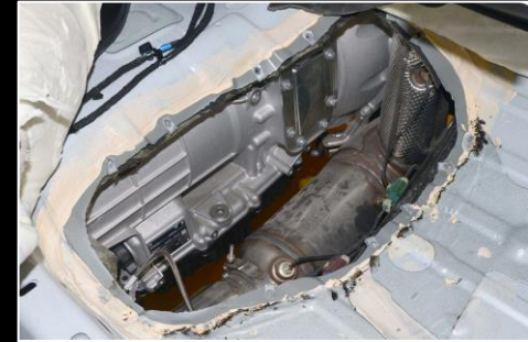
Patch Panel removed
