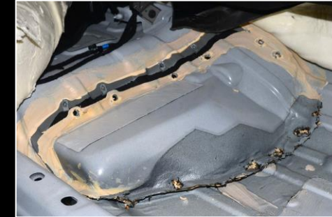
Patch Panel w/ Foot Pad
